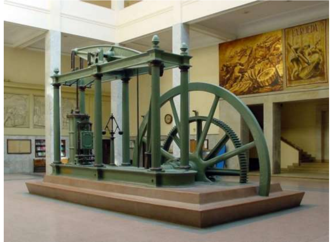
A late version of a Watt double-acting steam engine
